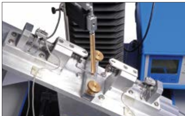
Fig 1 Experimental setup with an implant-abutment assembly embedded in an aluminum bar and positioned in a universal testing machine at a 30-degree angle to the long axis of the implant; the vertical brass-colored bar represents the load applicator. Mechanical probes are touching ( left ) the implant shoulder and ( right ) the abutment to transfer any movement to the remotely positioned extensometers.
